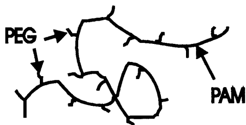
Figure 1 Schematic structure of long PAM having short PEG pendant chains to give a comb copolymer
