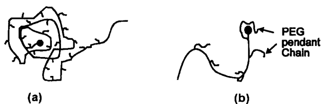
Figure 9 Schematic description of shielding effect on propagating radicals. (a) Radical shielded by a growing polymer chain, i.e. growing chain effect; (b) radical shielded by a pendant chain in the macromonomer, i.e. pendant chain effect
